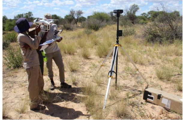
Figure 12. Equipment used for multispectral survey. a) DJI Phantom 4 Multispectral drone. b) DJI D-RTK 2 high precision GNSS mobile station (Zutshwa, 26/03/2024).
