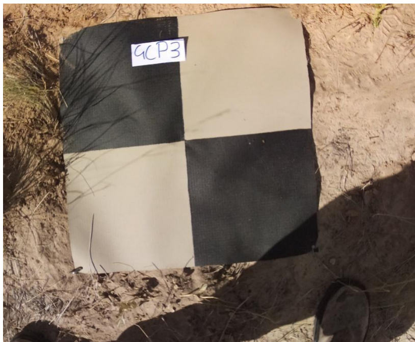
Figure 4. Brightly coloured canvas GCPs with black backgrounds enhance visibility and precision. The GCPs, measuring 50 cm x 50 cm, were constructed using brightly coloured canvas material with a black-painted background for enhanced visibility. The centre of each GCP was precisely measured using a DJI Phantom 4 multispectral drone, maintaining a 1 m altitude from the ground.
