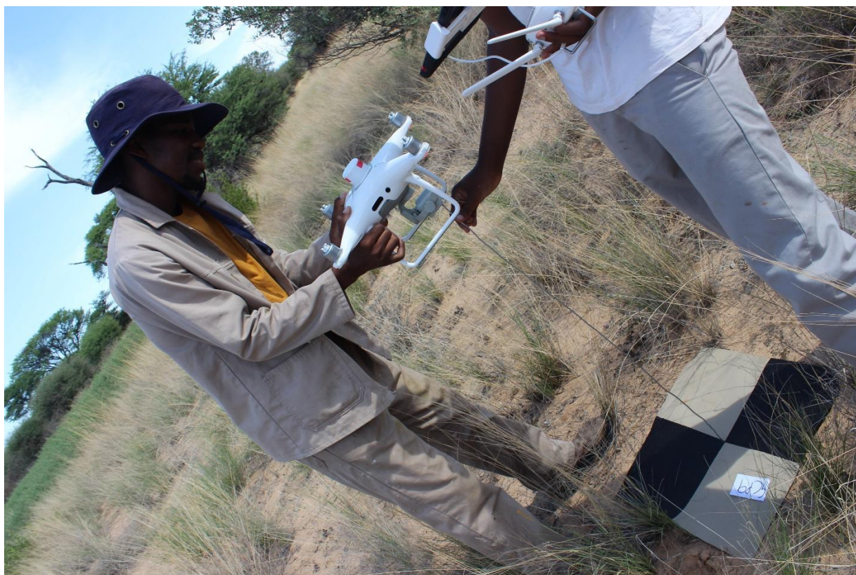
Figure 9. Geolocation of GCPs using the DJI D-RTK2 base and Phantom 4 multispectral rover system. This figure illustrates the process of geolocating GCPs with the DJI D-RTK2 base station paired with the DJI Phantom 4 Multispectral (P4MS) drone. A 1-meter-long rod was used as a height offset for the drone to have a consistent height measurement (Photo taken on 26/03/24).
