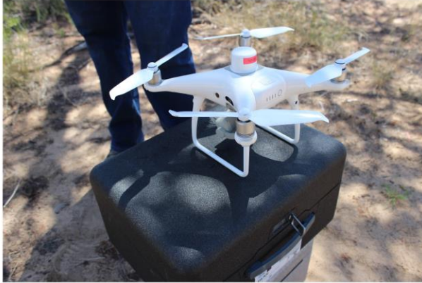
Figure 12. Equipment used for multispectral survey. a) DJI Phantom 4 Multispectral drone. b) DJI D-RTK 2 high precision GNSS mobile station (Zutshwa, 26/03/2024).
